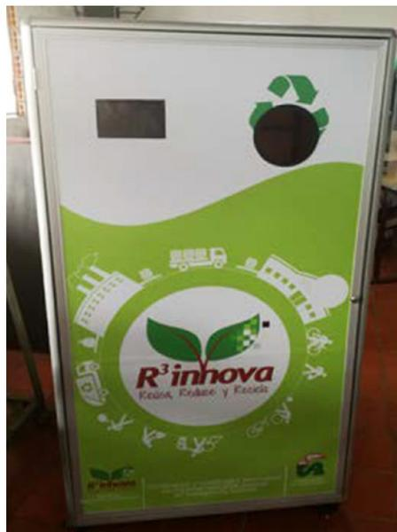
FIGURA 3. ESTRUCTURA EN ALUMINIO Y RECUBRIMIENTO EN PVC
