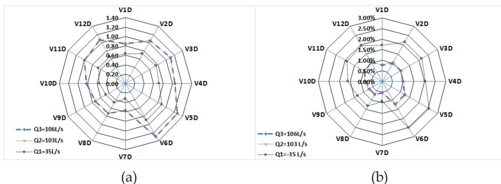
Figure 7. (a) captured flow rate (vertical column in the graph) for each version of the generator in mL / s and (b) Percentage of flow captured by 7-12 versions referred to versions 1-6.
