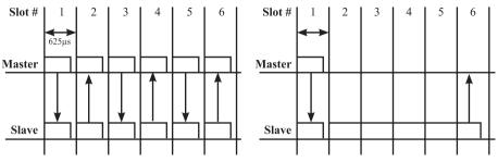
Figure 1. Transmissions of single-slot and multi-slot link packets
