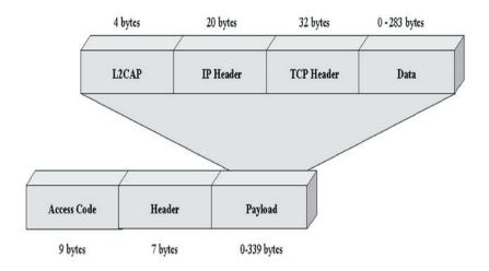
Figure 5. ACL link packet structure
